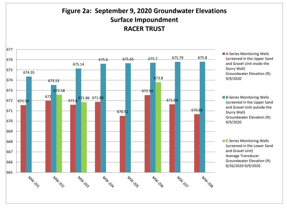
Note: Table 1 provides the groundwater elevation from the physical gauge data collected on September 9, 2020. Figure 2a presents the average transducer groundwater elevation for each C-series well.
