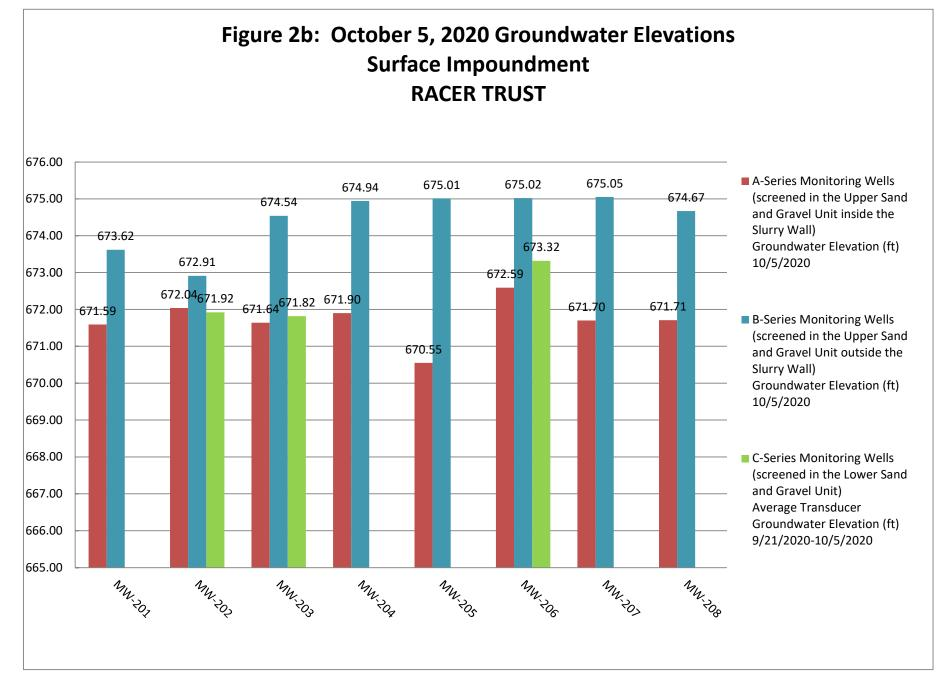
Note: Table 1 provides the groundwater elevation from the physical gauge data collected on October 5, 2020. Figure 2b presents the average transducer groundwater elevation for each C-series well.
