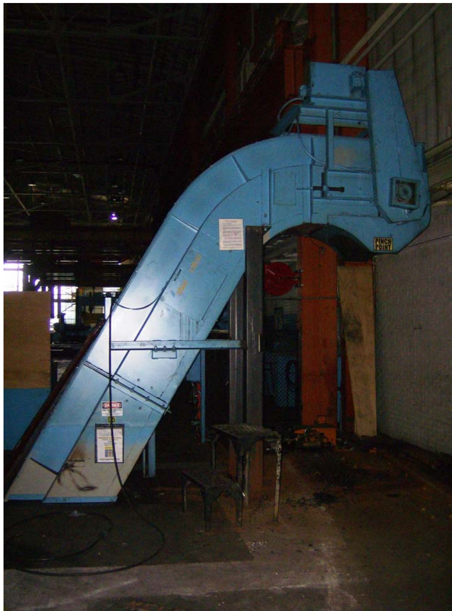
Photo 47: Grinding swarf conveyor
