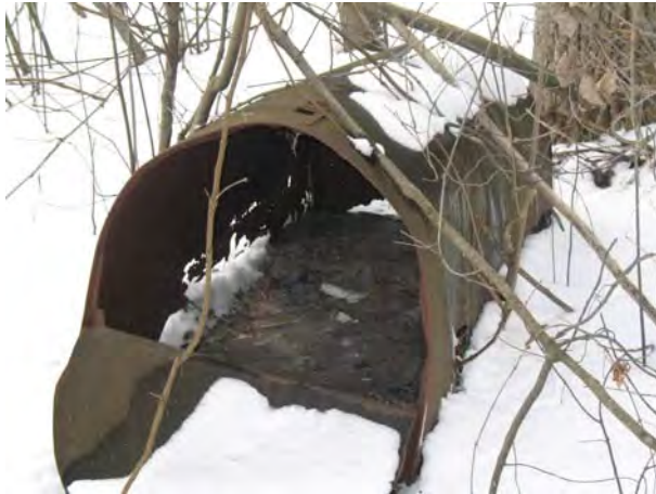
Photograph 8. View of an empty approximate 300-gallon AST located in the eastern portion of the Site.
