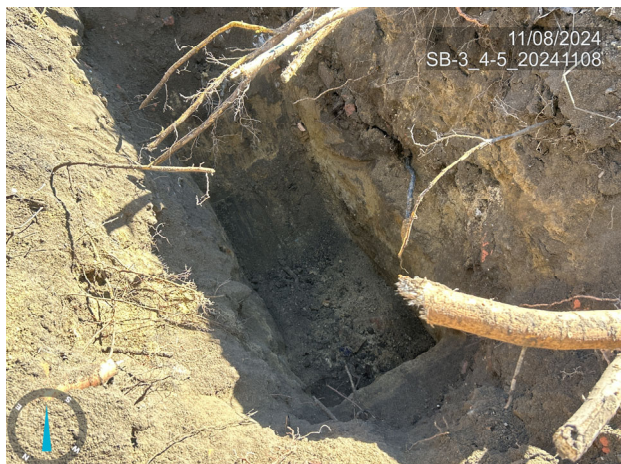
Test pit that was dug for gathering sample SB-3_4-5_11082024
