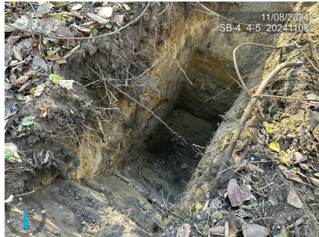
Test pit that was dug for gathering sample SB-4_4-5_11082024
