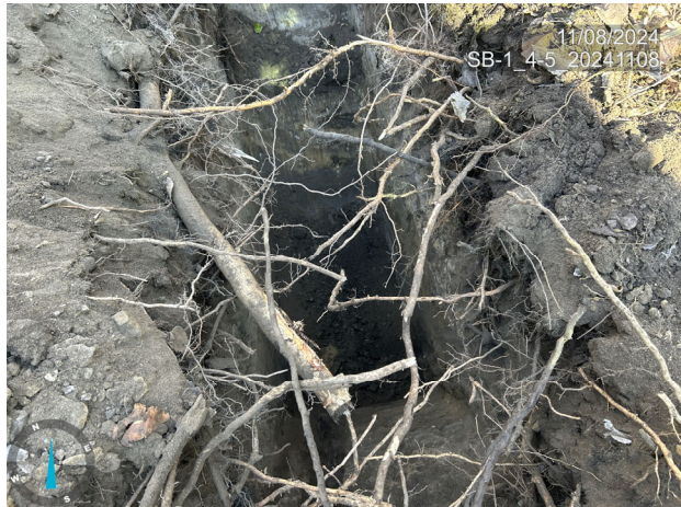
Test pit that was dug for gathering sample SB-1_4-5_11082024
