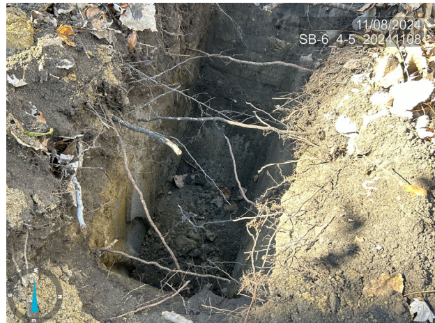
Test pit that was dug for gathering sample SB-6_4-5_11082024
