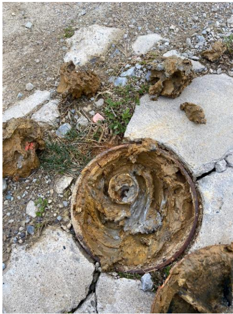
Photo 1: View of damaged monitoring well MW 76R-17
