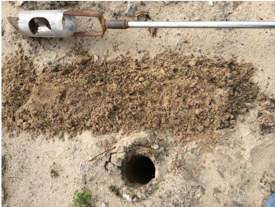
Photo 3 – View of SB324-14 boring and soil cuttings.
