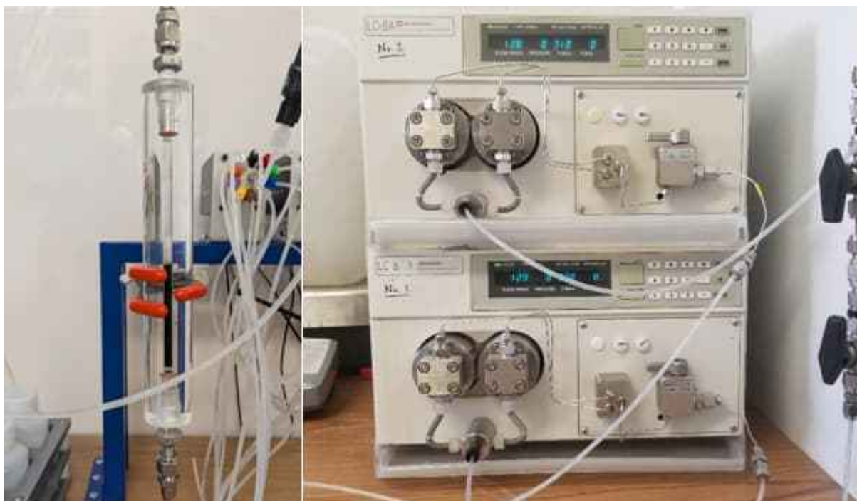
Figure 2: RSSCT column plumbed for operation (left) and RSSCT pump setup (right)
