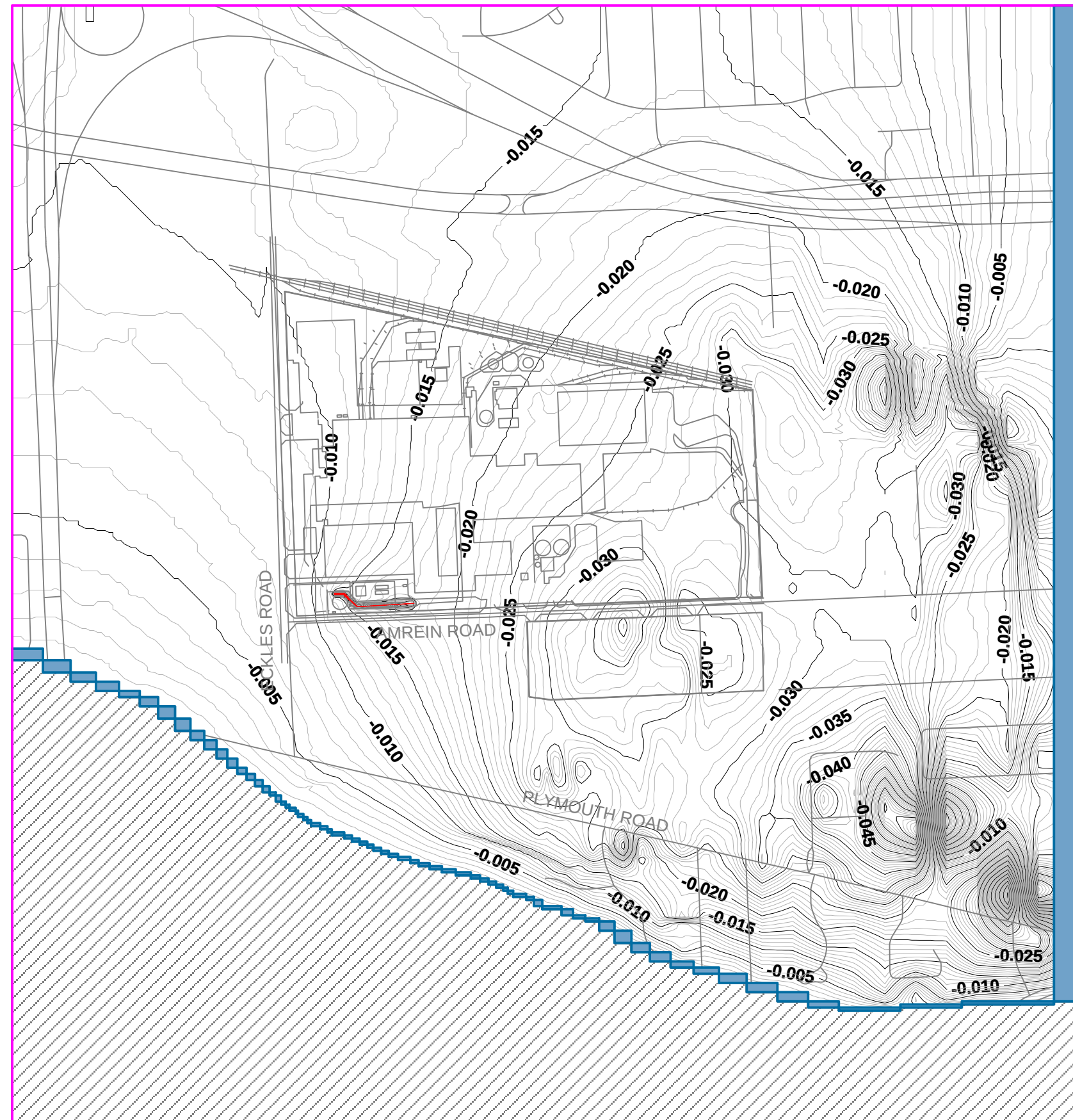
figure 4.4 GROUNDWATER FLOW MODEL - 8 LAYER MODEL GROUNDWATER ELEVATION DIFFERENCES 13000 ECKLES ROAD SITE Livonia, Michigan
