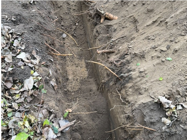
TP-106_0-2_11052024 No debris present
