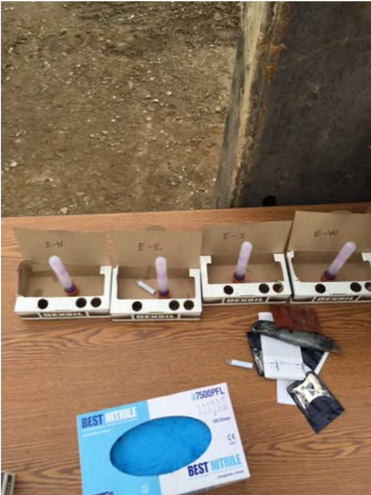
Field test kit results for excavation E – North, South, East and West sidewalls
